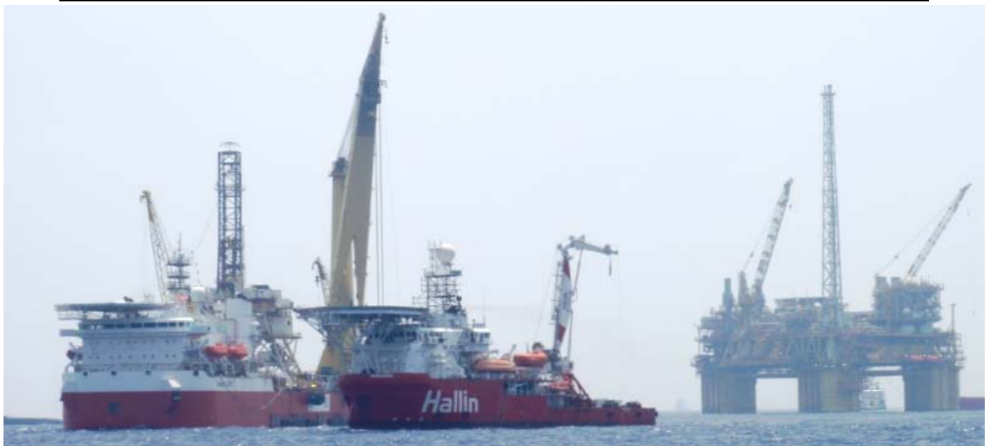
The DSV WINDMERE working close with the Sapura 3000 and the FPS Gumusut Kakap in the back ground. S3000 doing installation of mooring lines. Windermere equipped with 2x ROV for Survey work. Water depth 1400m
