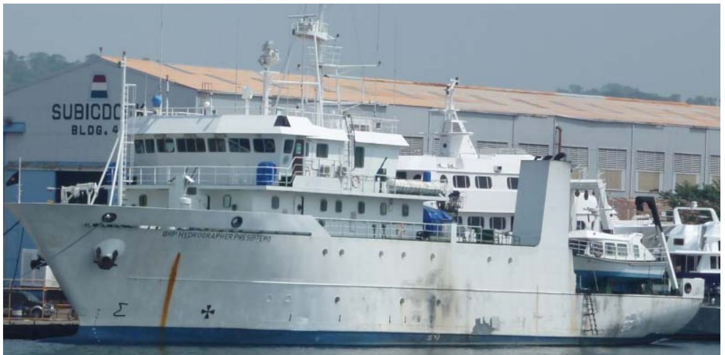
The Philippine Navy survey vessel BRP HYDROGRAPHER PRESBITERO moored at Subic Dock in Subic, the 1998 built vessel is having a length of 53.5 meters and a maximum speed of 13 knots was designed and built by Factories Vulcano in Vigo, Spain according to and under the close watch of Det Norske Veritas(DNV). Photo : Piet Sinke ©
