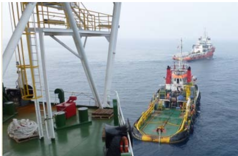
The AHTS RED FISH 4 takes over the towing gears from the LEWEK GRIFFIN whilst holding the FPSO Perisai Kamelia Photo's: Capt . Richard Leistra (c)
