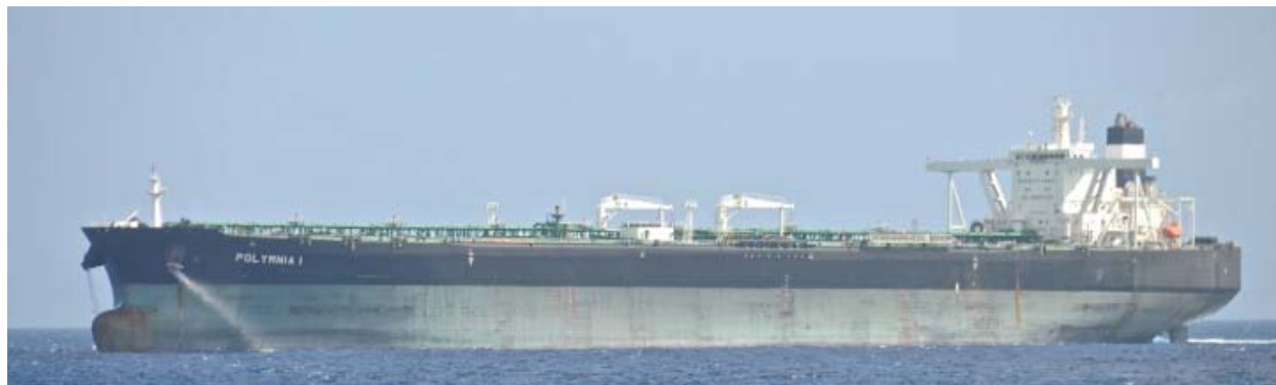
The crude oil tanker " POLYMNIA 1 ", which was June 24th, near Curacao, waiting to go to Bonaire. Her dwt is 296.812., l.o.a. 330 mtr, breadth 60 mtr and IMO nr is 9575955 Photo : Aart van Essen (c)
