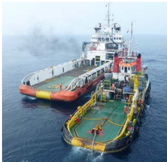
The AHTS RED FISH 4 takes over the towing gears from the LEWEK GRIFFIN whilst holding the FPSO Perisai Kamelia Photo's: Capt . Richard Leistra (c)
