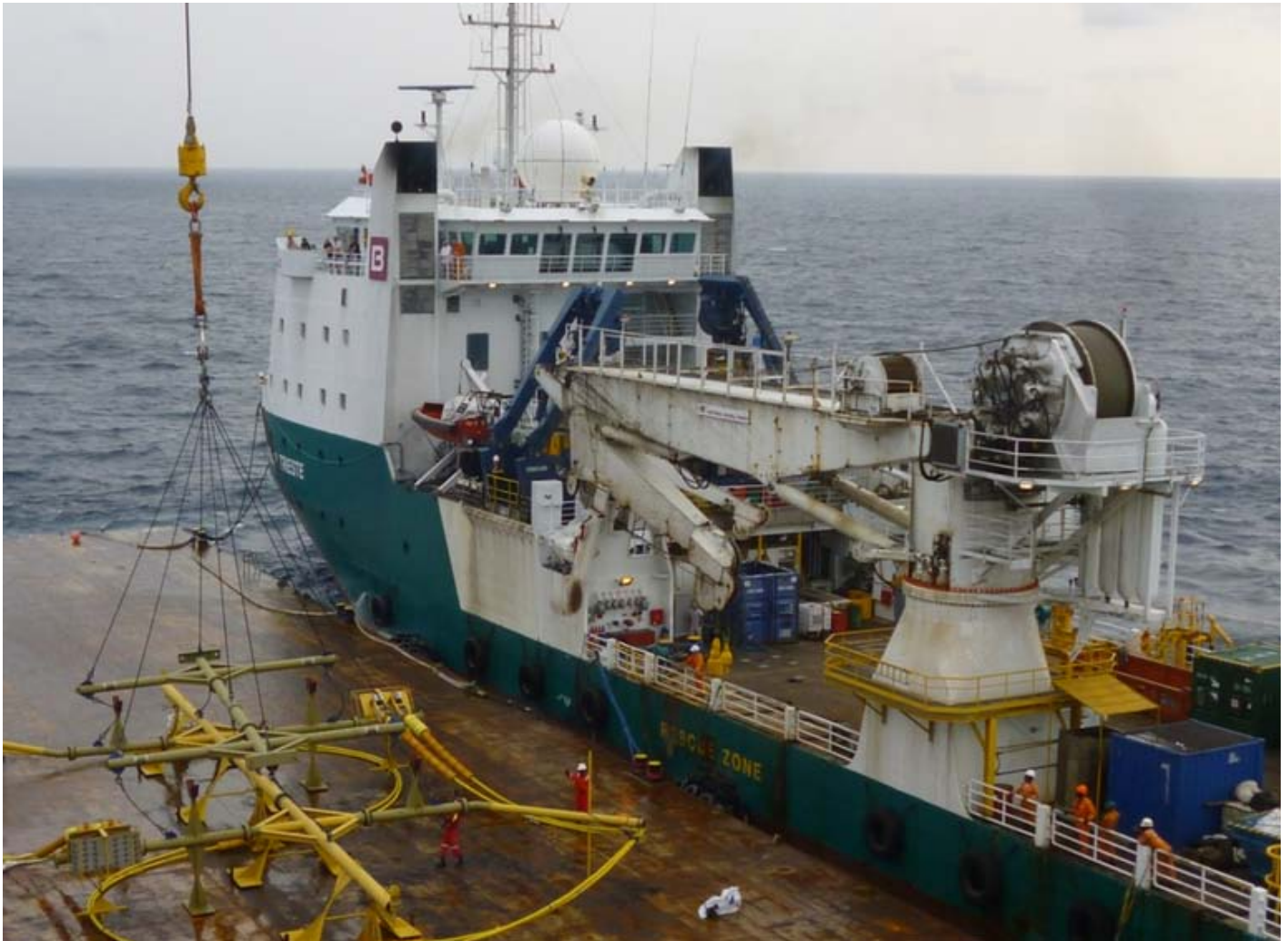
Bourbon Evolution 802 is taking strongback frame with subsea equipment from barge hold by Bourbon Trieste . Photo : Capt. Artur KAMINSKI – Master BOURBON EVOLUTION 802 ©
