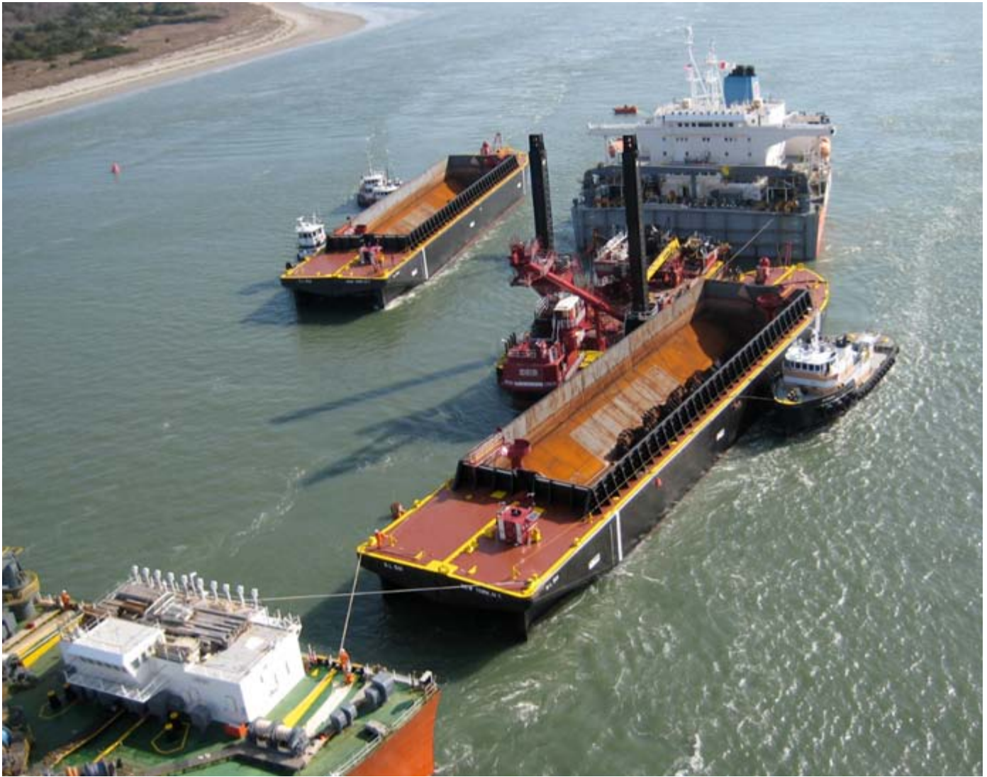
Dockwise HLV " TREASURE " in the process of loading dredging equipment at Charleston SC USA. Photo : Kees Kuyper ©
