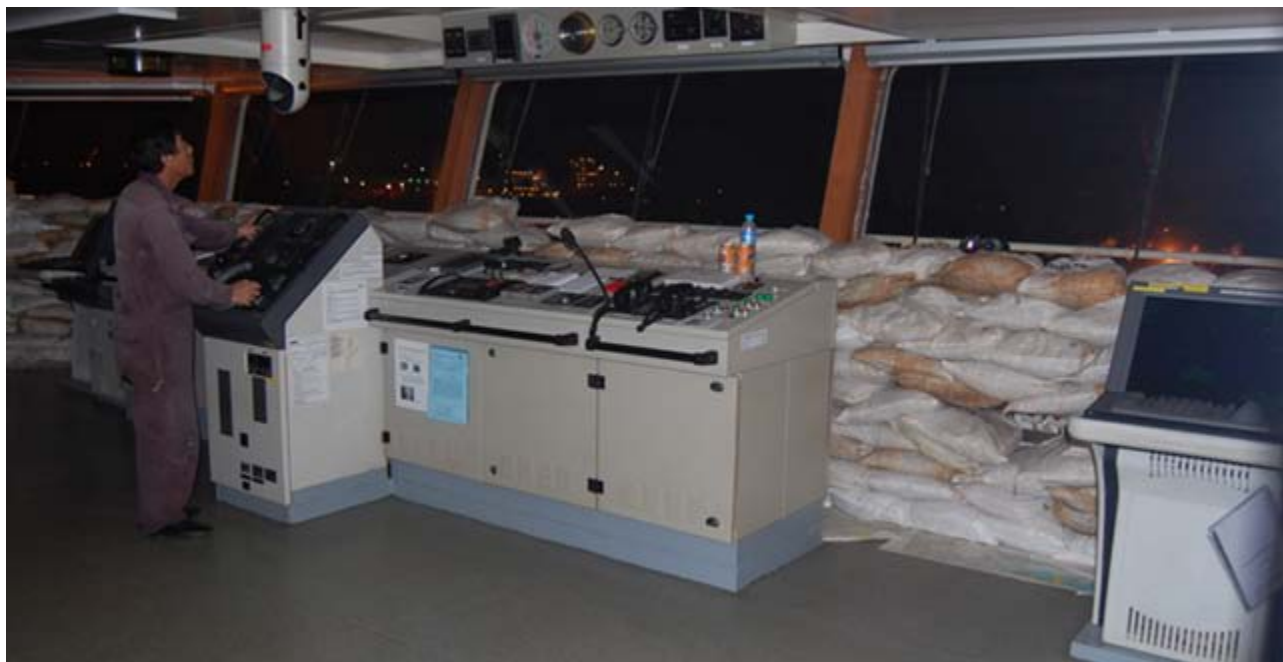
The wheelhouse of the OCEAN TIARA , with sandbags positioned on the inside to absorb / stop the bullets from pirates if the bullets come through the steel of the superstructure – Photo : Rik van Marle ©
