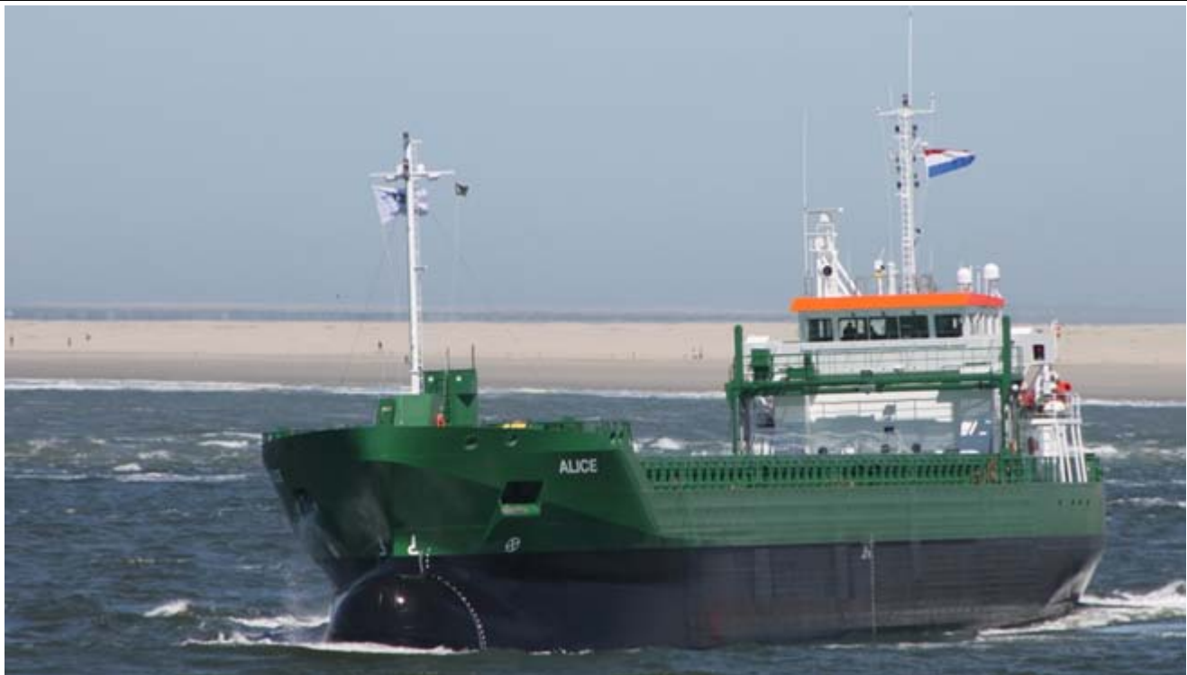
The newbuilt "ALICE" during a "hard to port" test off Borkum as seen from the Union Princess. Photo : Crew Union Princess (c)
