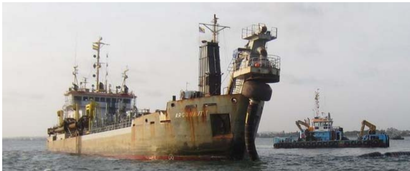
ARGONAUT pumping first load of sand through new sinker line. Next to it the JIFWORKER who positioned the pipeline. - Photo : Ernest van Arentsals (c)
