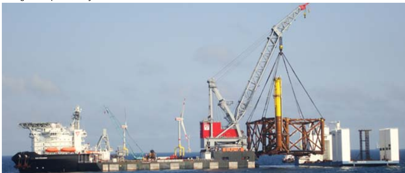
The OLEG STRASHNOV from Seaway heavy lifting, lifted a jacket from the Eide barge 33 at the Bard windfarm project in the North sea. Photo : Crew Union Princess ©
