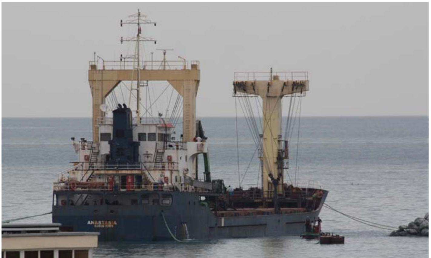
The mv ANASTASIA loaded with rock for the breakwater construction at Sochi Port, Russian Federation, being prepared for discharging the rock by means of an on-board excavator with long reach. Photo : Dirk van Uitert (c)
