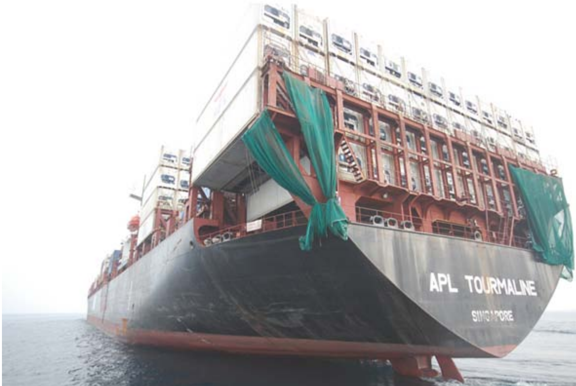
The APL TOURMALINE in the Port of Sohar (Oman) equipped with anti-piracy curtains Photo : Rik van Marle (c)
