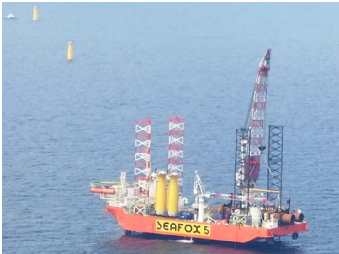
The 151m jack-up vessel Seafox 5 , spotted in the German bight - Northsea on may 29th, 2013, to install 80 monopile foundations at the 288MW DanTysk offshore wind farm. Photo: Cor Draijer ©
