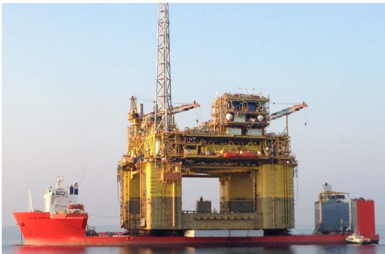
The FPS Gumusut Kakap loaded onboard Dockwise BLUE MARLIN off Johor (Malaysia)
