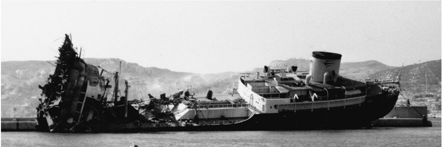
On 22/5/67 the 16,870tdw Liberian tanker CIRCE was en route from Sete to Naples in ballast when an explosion broke her in two and 38 crew died. The aft part was towed to Marseille where the above photograph was taken on 27/7/67. Photo : Maurice Napier ©
