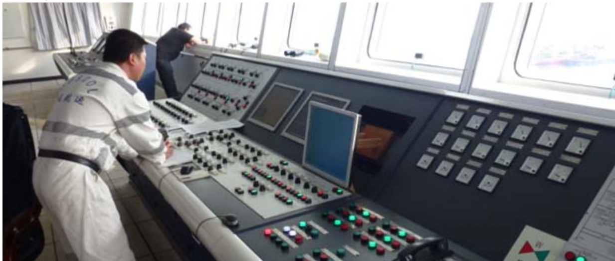
Top Ballast control panel at the aft section of the wheelhouse during the ballasting operation
