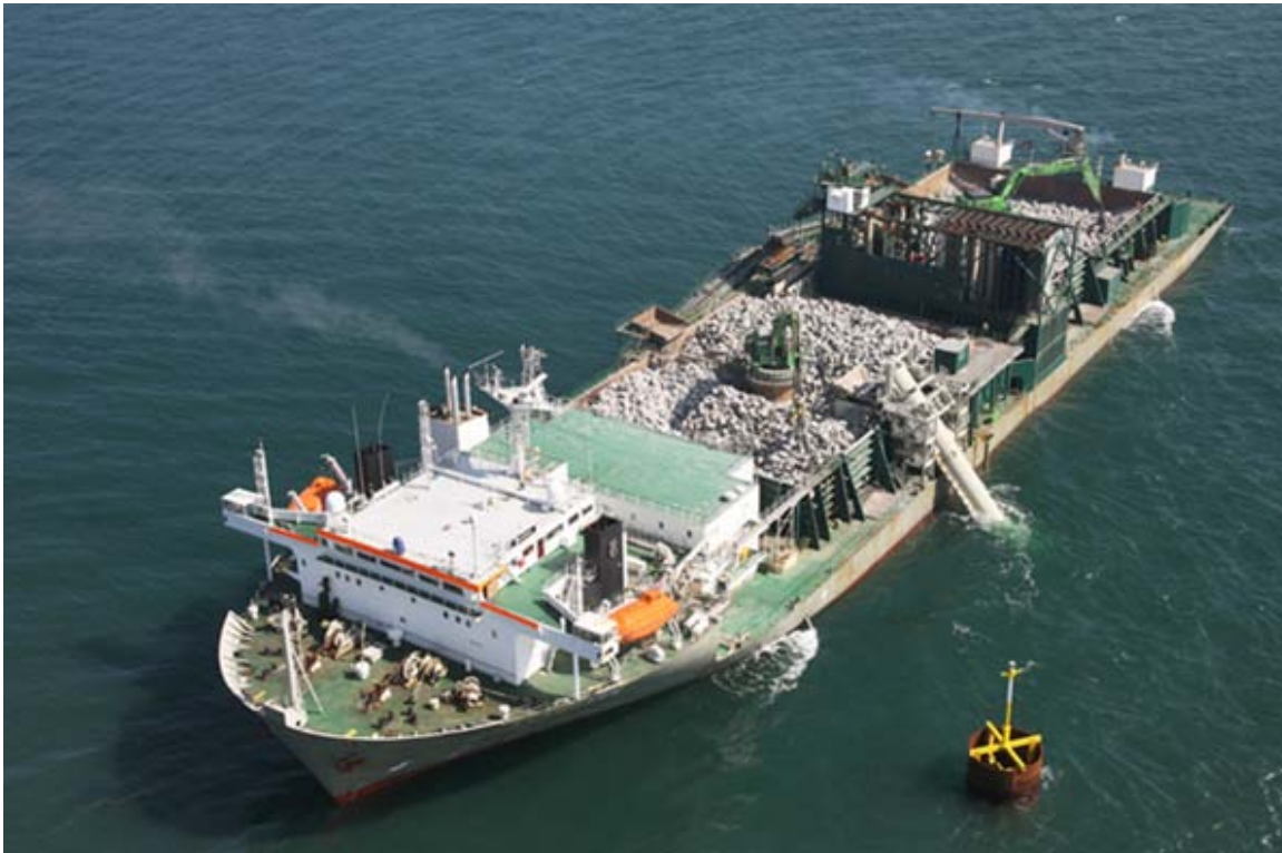
Tideway's SEAHORSE during Stone/ rockdumpng at the Meerwind project
