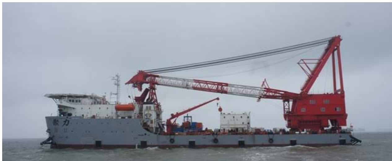
The Chinese crane vessel JU LI anchored at Shanghai anchorage, owned and managed by Shanghai Salvage Company . After installing Rolls Royce thrusters and a Navis DP-2 system the JU LI is due to execute DP trials.
