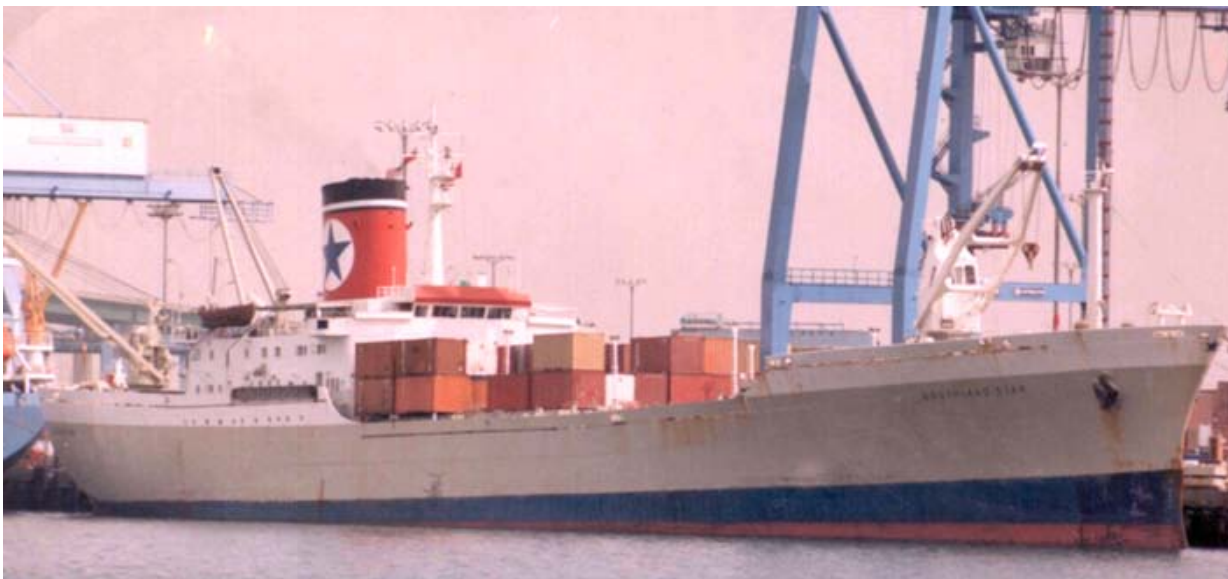
"SOUTHLAND STAR" moored San Predro, Los Angeles, in 1985 just after the maker of the photo: Brian Thornborrow left the vessel . If Brian remembers correctly The SOUTHLAND STAR was the first UMS vessel in the British Merchant Navy. She was built as a conventional refrigerated vessel and then converted to a refrigerated container vessel. She was a good ship, but the milk chocolate coloured lifeboats were always a puzzle, they did not stand out too well in the water, her sister vessel Wellington Star . also had the same coloured lifeboats, Photo : Brian Thornborrow ©
