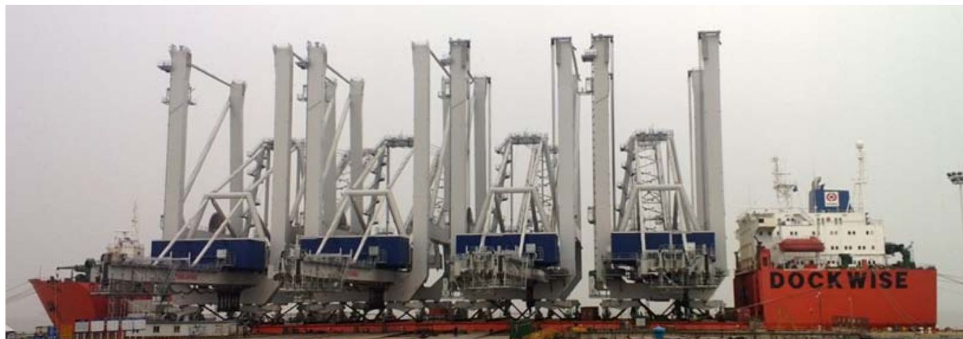
TEAL of Dockwise , loaded with four super post Panamax container cranes at Nantong, China. The top sides of the cranes are lowered for safe passage of the Sutong Bridge over the Yangtze River.
