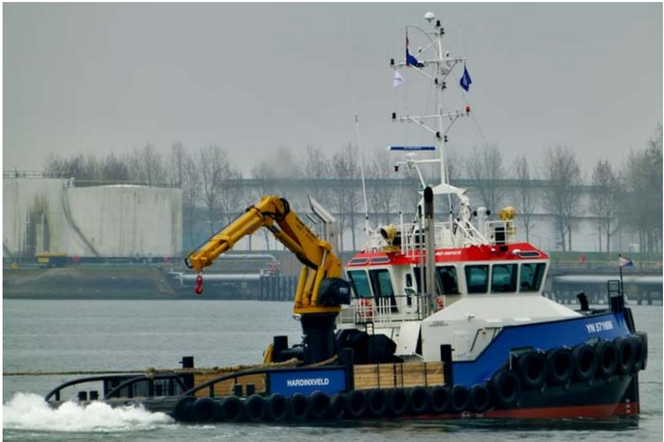
The Damen built Shoalbuster 2709 with yard number 571686 during bollard pull tests yesterday in Rotterdam Caland Canal – Photo : Jan Oosterboer ©
