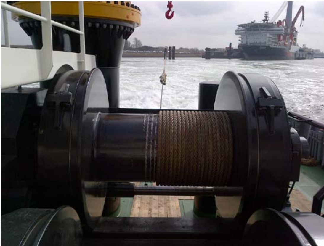
A DMT reversed ANCHOR-HANDLING WATERFALL WINCH during trials in Rotterdam, on board of the DAMEN Shoalbuster 2709 vessel with YN571686 (with HEEREMA's ÆGIR in the background). – Photo: Lars Herweijer – DMT ©
