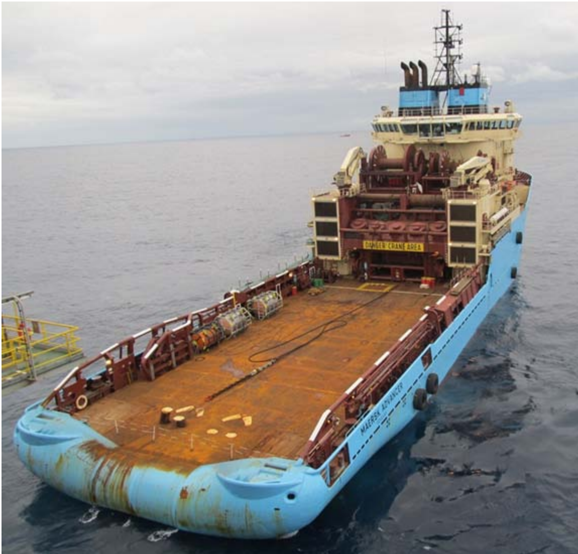
280 BP MAERSK ADVANCER conducting a test approach for the towing bridle of the DP drilling rig Pride Portland at Espirito Santo Basin – Brazil Photo : Auke Ruijg. (SDPO)
