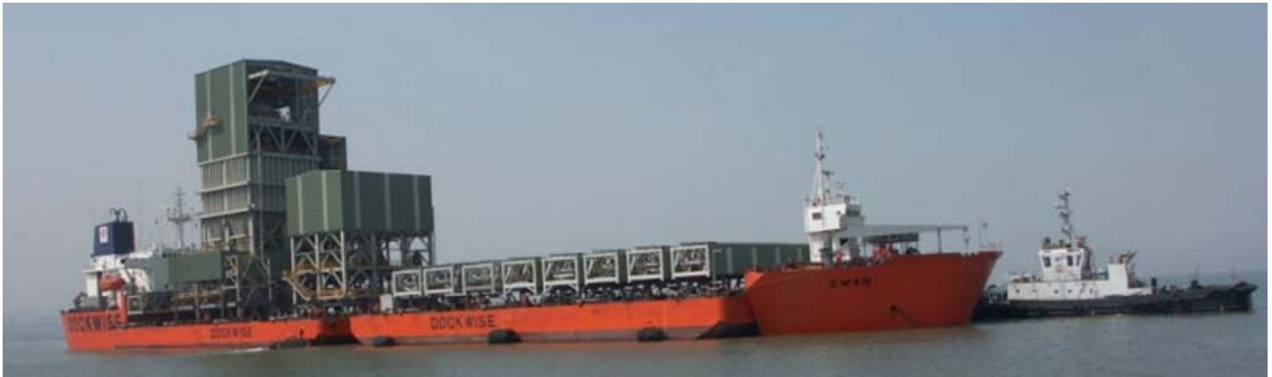
Dockwise SWAN is loading modules at the Penglai east harbor anchorage by floating on their newly built "super pallet barges (60 m x 40 m)". The modules are built at PJOE [ Penglai Jutal Offshore Engineering ] with destination Australia. Photo: Tingting Zhao (c)
