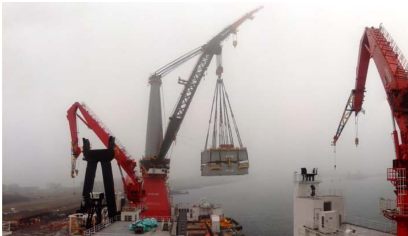
Heerema's new DCV Aegir seen performing single hook load tests on the main 4000mT crane.
