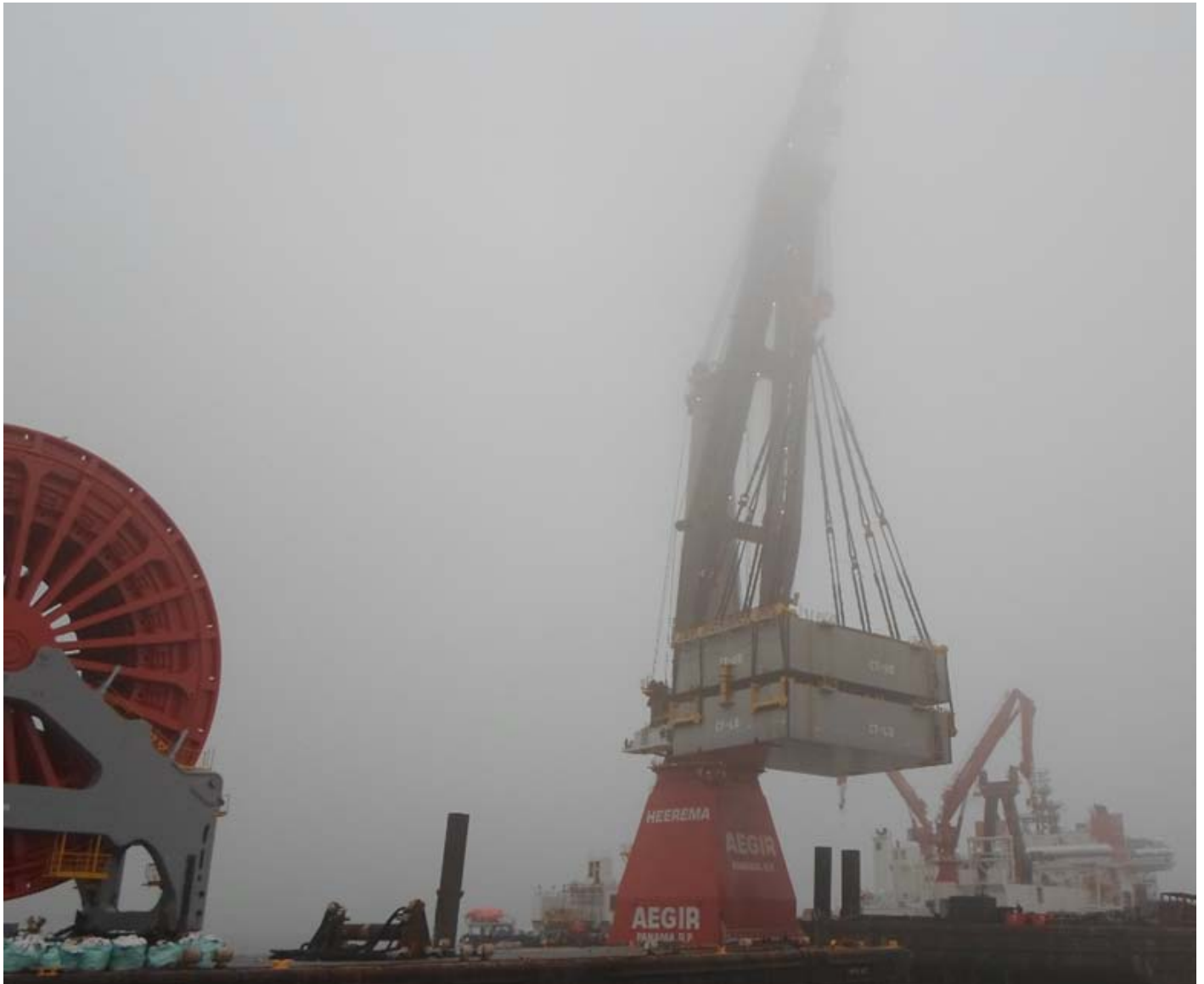
"A foggy morning in the Rotterdam Calland canal. Heerema's new DCV Aegir seen performing single hook load tests on the main 4000mT crane. Alongside the Aegir the Heerema barges H-114 and the MWB-403 which is having the pipe reel parked on its deck" - Photo : Bram van Koert ©
