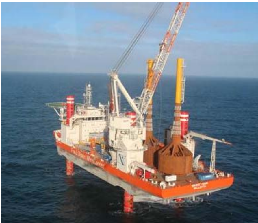
The BRAVE TERN installing Meteorological Masts at the Dogger bank (Northsea) – photo's : Crew Brave Tern ©
