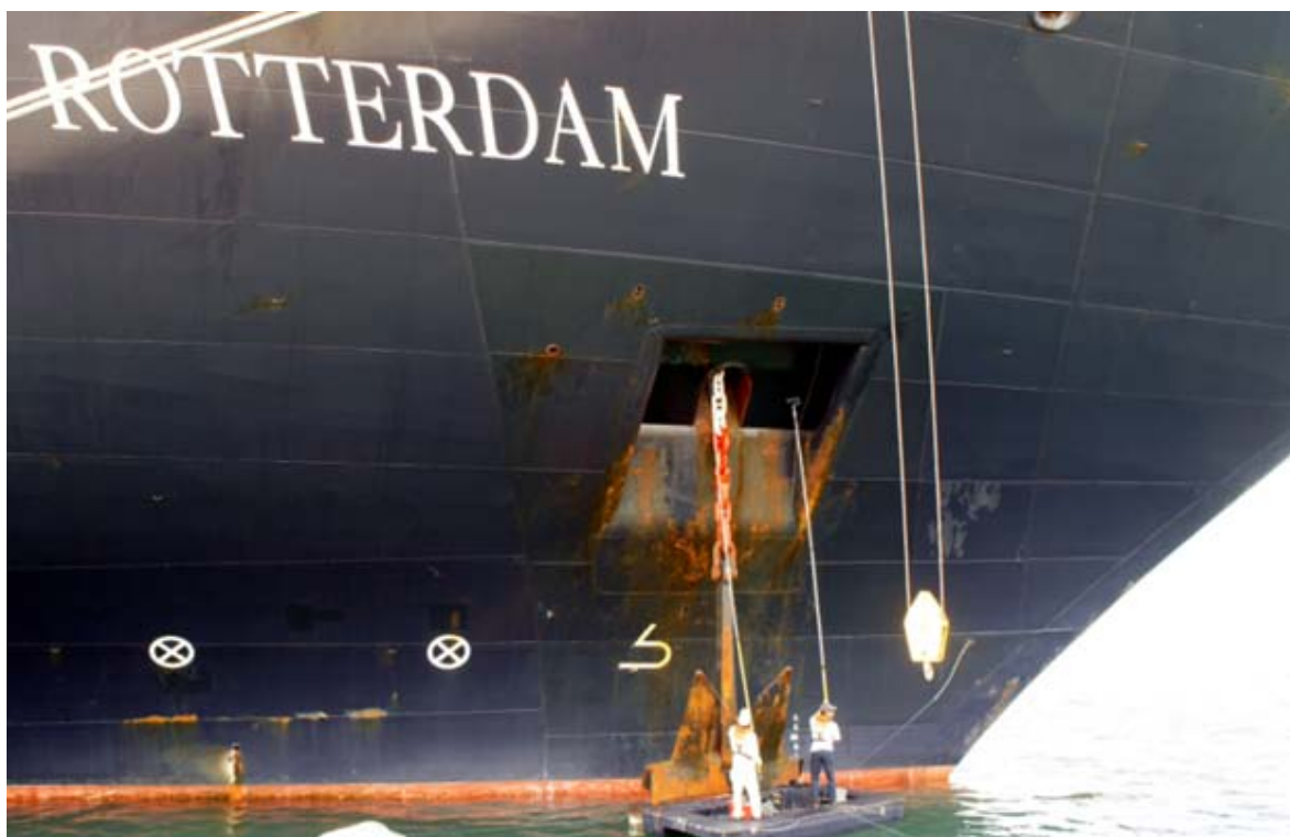
Maintenance done on HAL's ROTTERDAM SB Anchor whilst moored in Port Rashid (Dubai)
