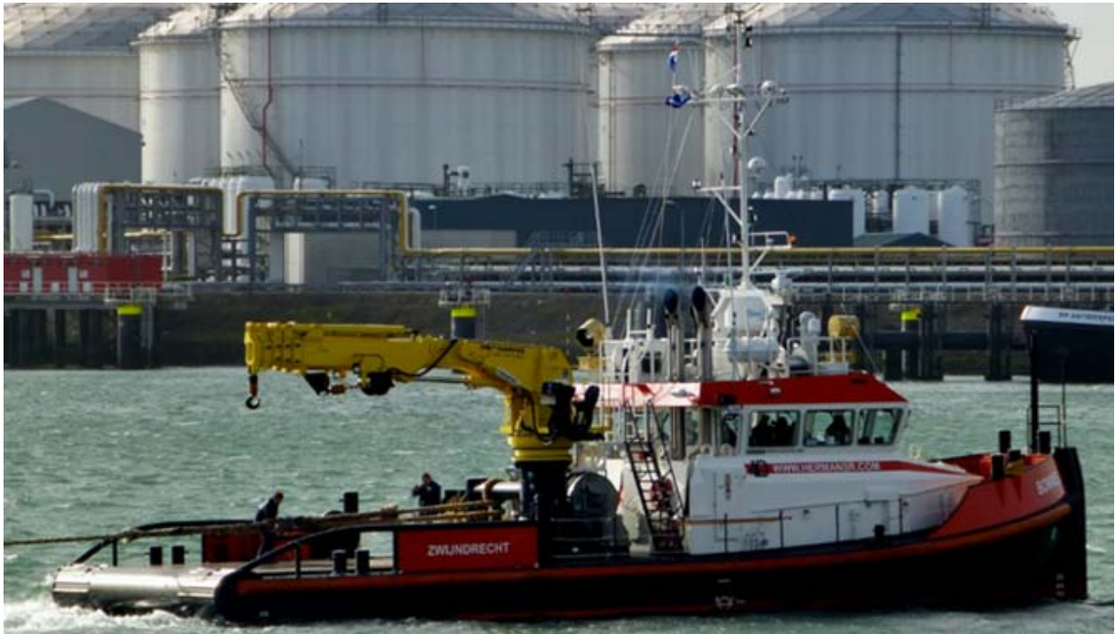
The DAMEN Shoalbuster 2509, BOMMEL during bollard pull tests in Rotterdam-Caland canal – photo : Jan Oosterboer ©
