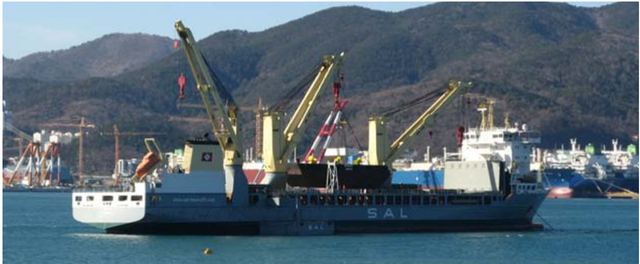
SAL's "MV TRINA " seen in Okpo (DSME) harbor offloading the test pontoon for the load tests of the 4000mT main crane of Heerema's newbuild "DCV AEGIR ". Photo: Wouter Blom ©
