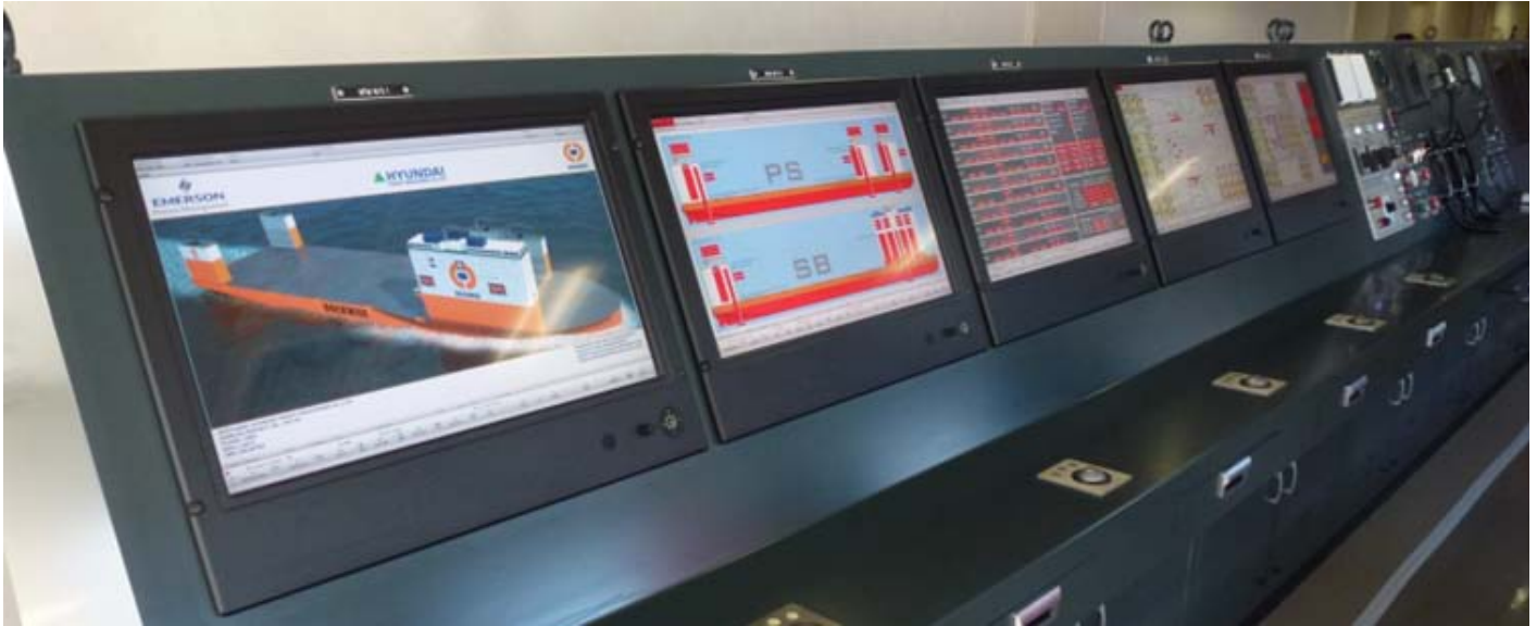
The ultra modern Ballast panel with all large (27 ") touch screens in the ballast control room
