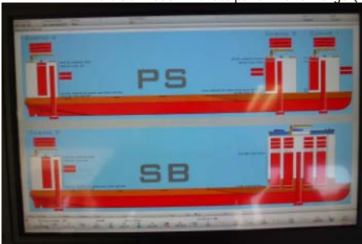
The ultra modern Ballast panel with all large (27 ") touch screens in the ballast control room
