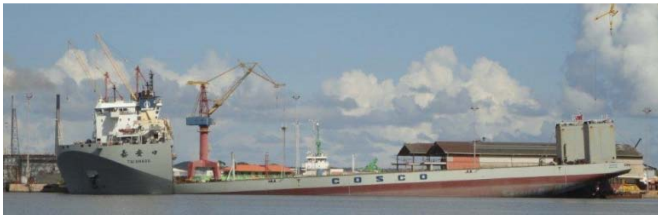
05-12-2012 : TAI AN KOU trimmed over the bow for PS/STB Azipoth repairs at the Curacao Dry-Dock Company Ltd, Photo : John Smit ©
