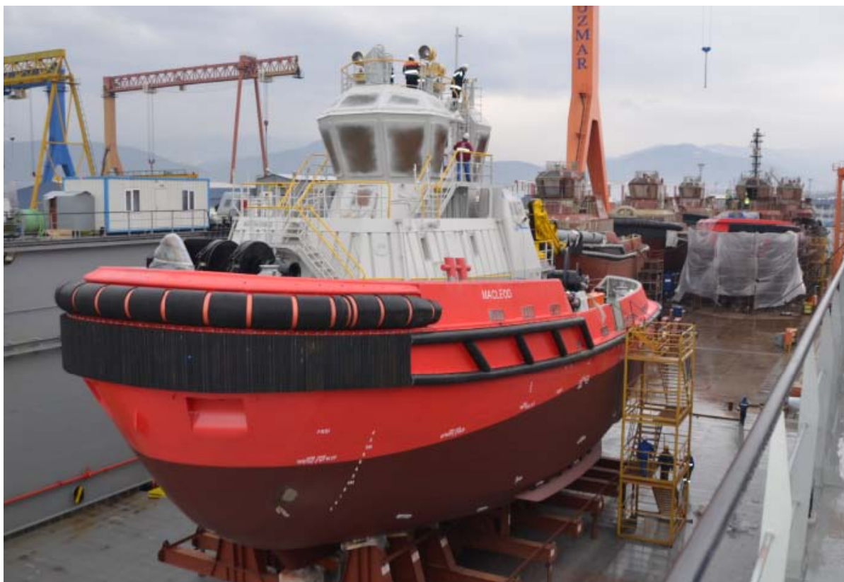
Seen at Uzmar Shipyard in Turkey last Wednesday, Rio Tinto's new Robert Allan design 60 ton bollard pull ADS tug MACLEOD for the Cape Cuvier operation in Western Australia in the floating dock before launch. Length 30.8m, Breadth 12m and a draft of 5m. – Photo : Carl Jernert ©
