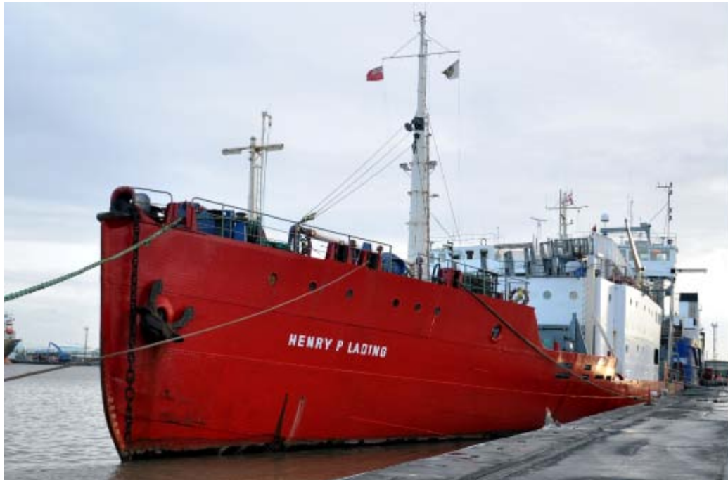
The 81 year old hull of the Henry P Lading . Photographed in Immingham dock 28/12/11. Originally Built as the oil tanker Peter Hurle in 1930 and re-named Esso Kobenhavn in 1948. She was scrapped in 1963 in Odense, but the fore section was converted into a cable/pipe laying barge.
