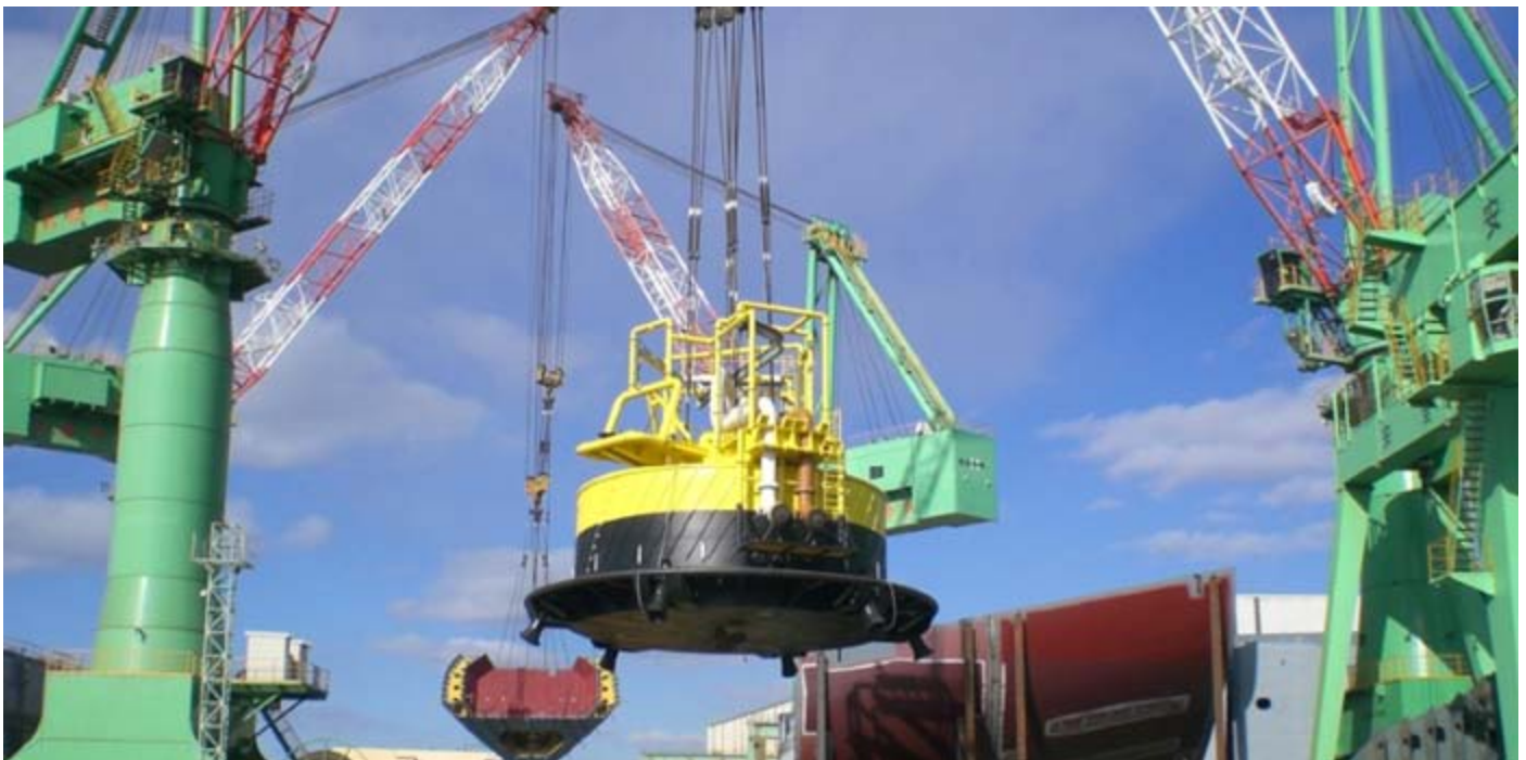
SBM CALM buoy (weight : 275 Ton) being air lifted to be lowered in the water at the DSIC Yard Dalian China for final ballasting and trimming purposes. - Photo : John Ravenshorst ©
