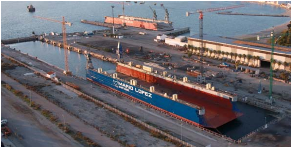
Above seen the Floating Dock “ Andalucía ” owned by Mario López Shipyard (Cernaival Group) once her lengthening of 45 mtrs has been completed (New length 145 mtrs). Photo : Cernaival Shipyard ©
