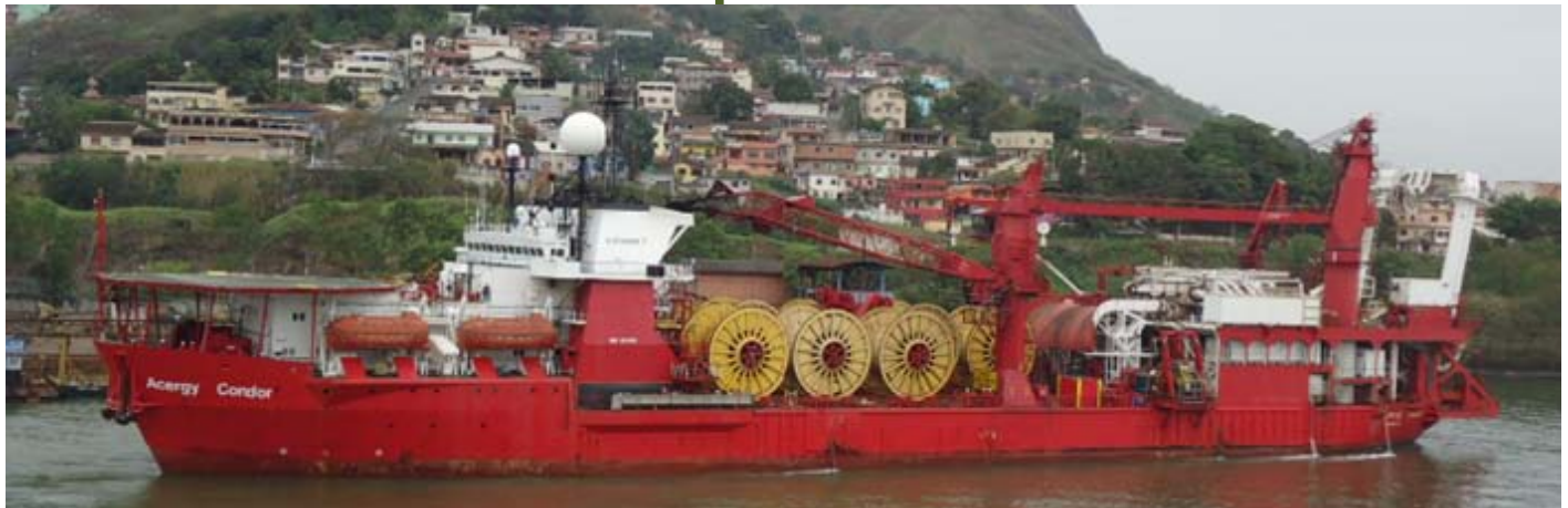
The ACERGY CONDOR seen backing up towards Bavit spoolbase in Vitória, Brazil to load flexibles. Photo : Mick Edses – Normand Seven ©
