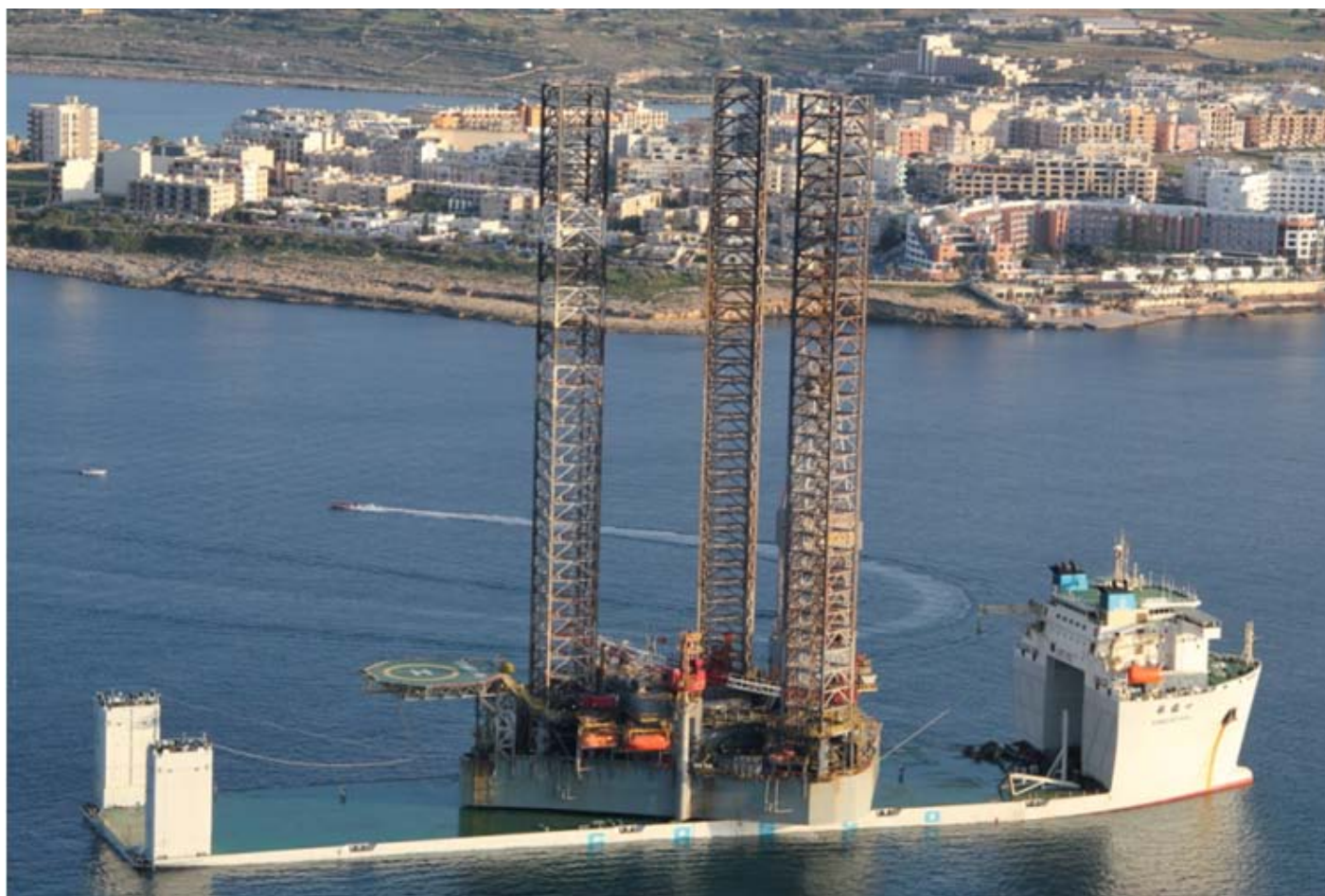
Above seen the 2011 built semi-sub heavy load carrier XIANG RUI KOU loaded with the jack up oil rig ENSCO 85 at St. Paul's Bay, Malta on Saturday 3rd December, 2011.
