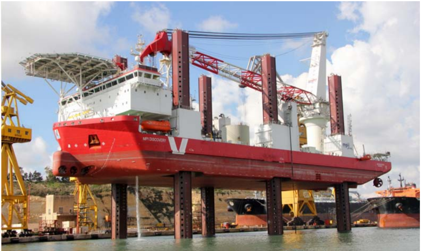
Above seen the MPI DISCOVERY jacked up 17m from sea level during trials at the Palumbo Malta Shipyard Ltd , Grand Harbour, Malta on Sunday 4th December, 2011.
