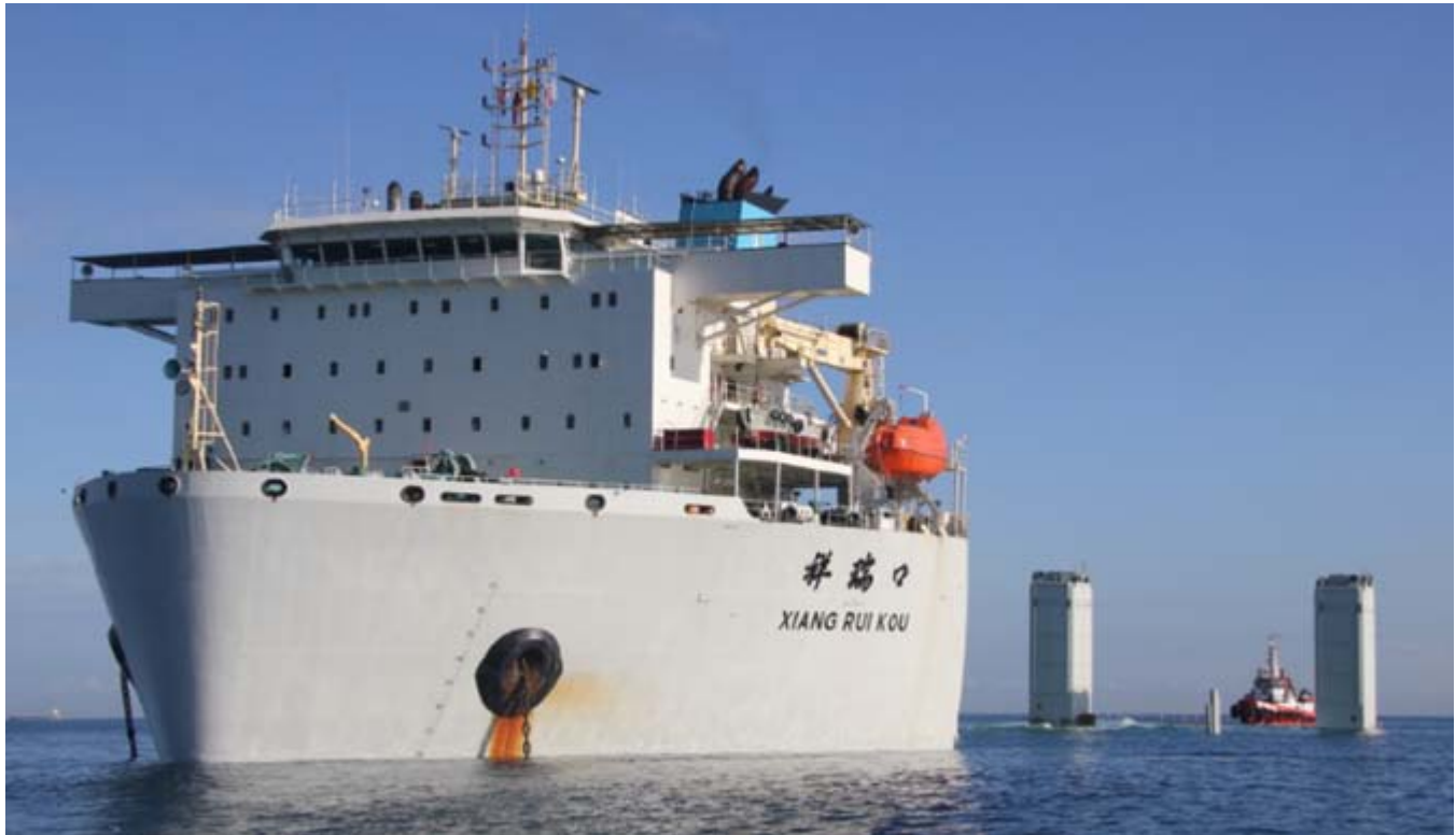
Above seen the 2011 built semi-submersible heavy lift ship XIANG RUI KOU at St. Paul's Bay, Malta submerged on Thursday 24th November, 2011 for ENSCO 85 lifting operation.
