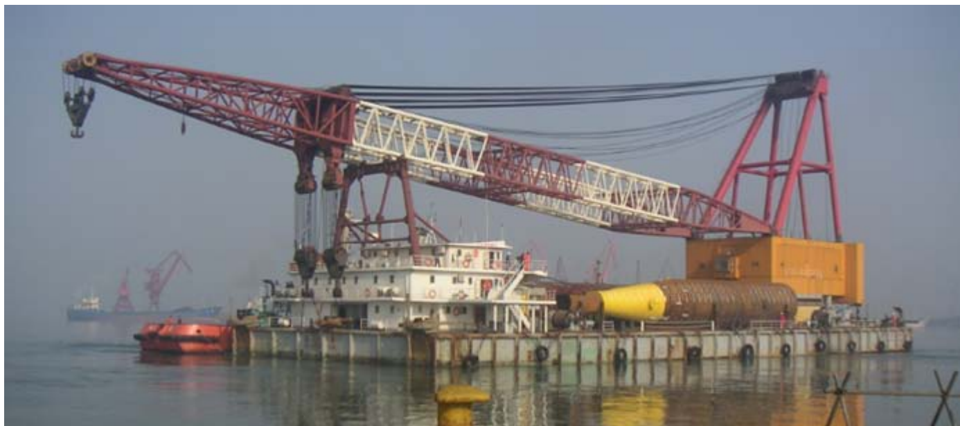
The derrick barge " SulianHai QuiZhong II " has just collected two windmill foundation monopods from the PJOE yard in Penglai for installation in the Bohai Bay, North East China. The derrick barge is fitted with a China made 1,000 Ton revolving crane. – Photo : Tony Schenk ©
