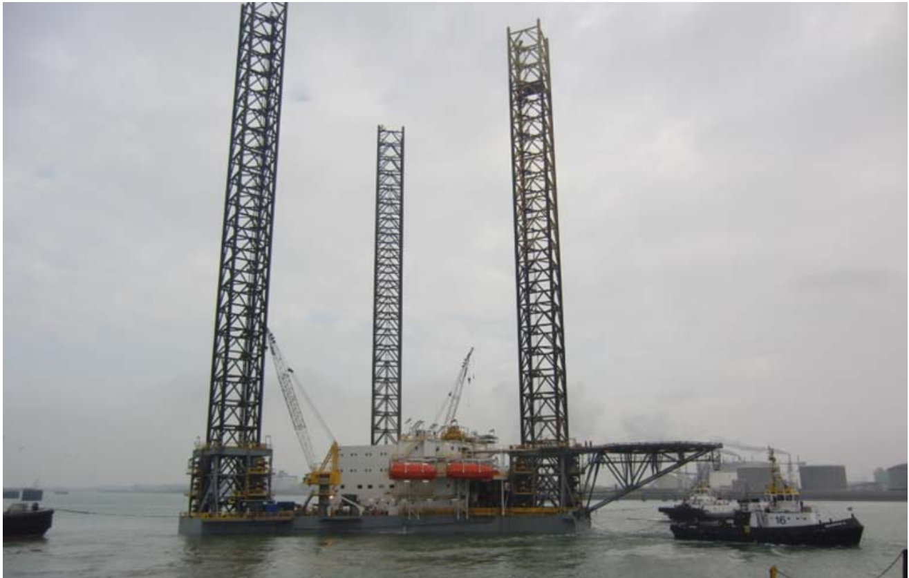
The AMS rig ATLANTIC LABRADOR leaving the Scheldepoort yard after a 4.5 months conversion from drilling into a accommodation unit. Photo : Klaas Bosma ©
