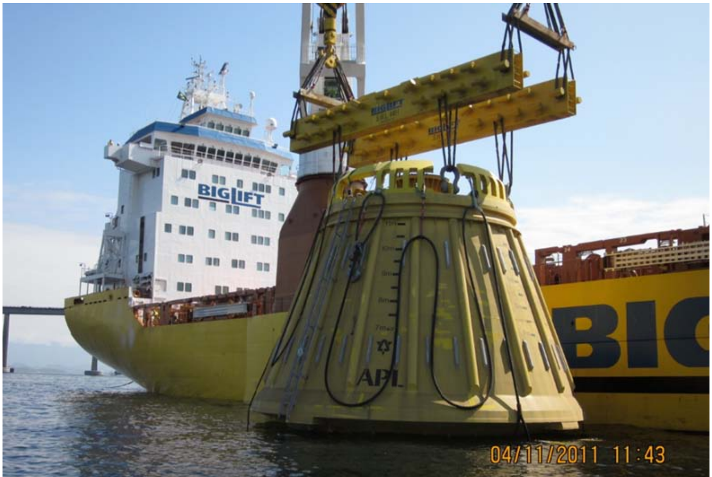
The FPSO OSX-1 mooring buoy seen being discharged in Rio de Janeiro. Happy Dover discharged the buoy with a height of approximately 17 meters, diameter of 14 meters and weighing over 700 tons by her own cranes.
