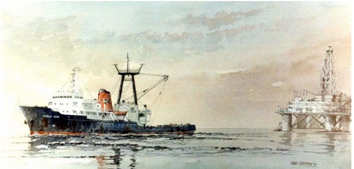
Watercolor from Hans Breeman made in 2001 of a nice shaped Tug from International Transport Contractors (ITC) , mv Sable Cape . Total Horse Power 9000 bhp, max speed 13,7 knots, 1524 grt, Bollard pull: 110 tons. www.hansbreeman.nl
