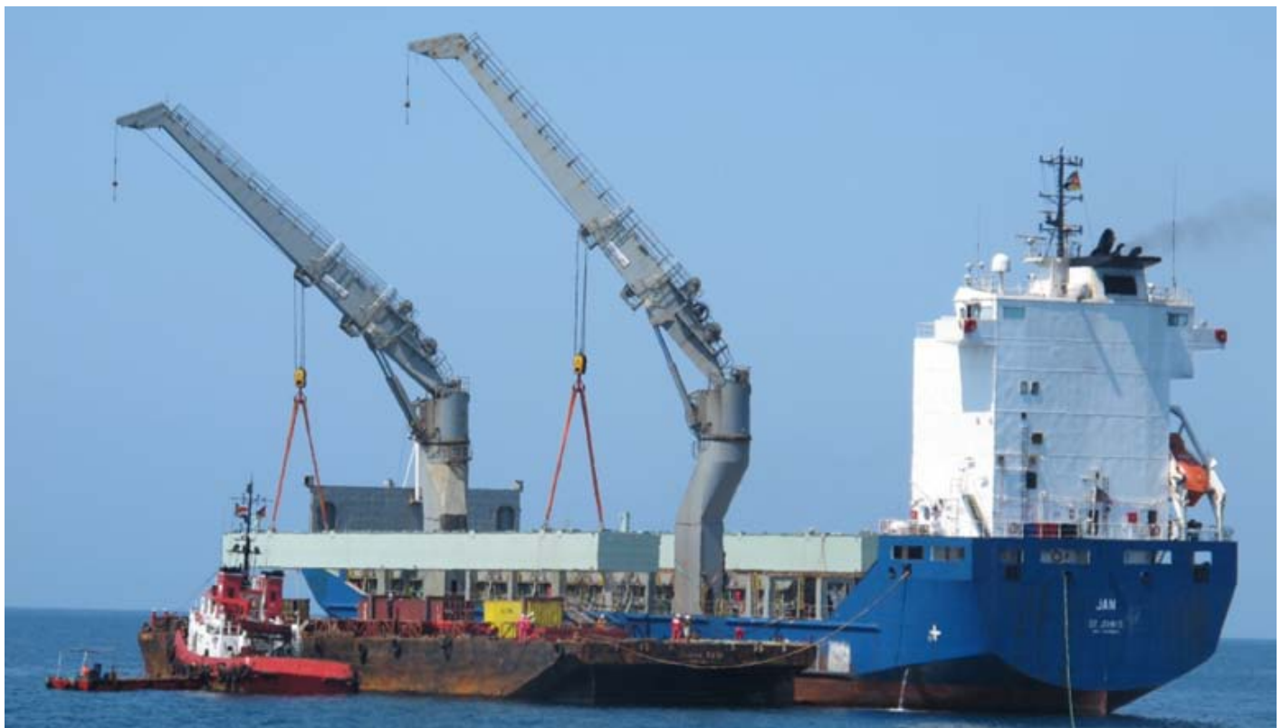
COMARCO transshipping with tandem lift 49 meter long, 100 ton pontoon sections from MV Jan to Comarco barge 231 offshore Malfamede Island, Mozambique. The pontoons to be landed ashore at the exposed beach for the MOMA sands mining expansion project. Photo : Philip Fay - www.comarconet.com ©
