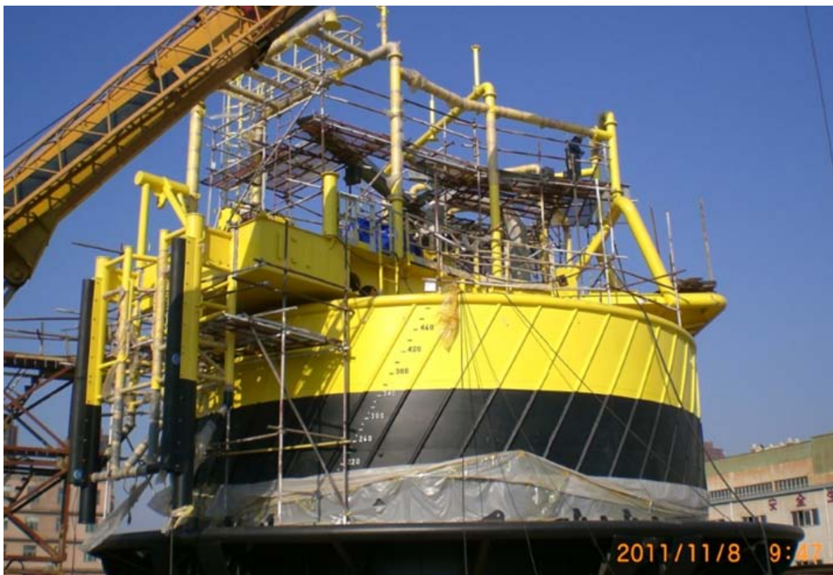
The fabrication of a SBM Offshore CALM buoy at the DSIC shipyard Dalian ,China for Tanzania
