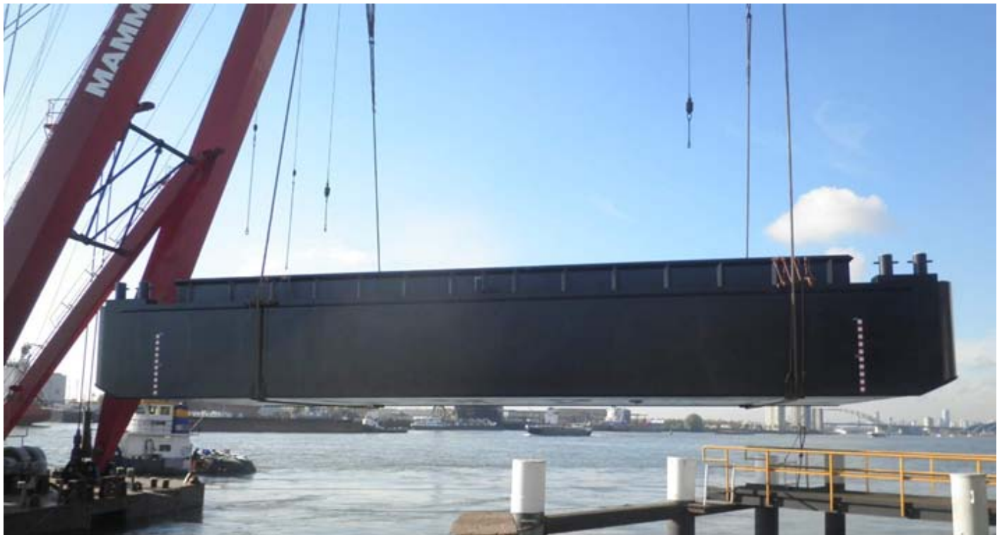
The first of two fenderbarges for Marcor Stevedoring B.V. in the Waalhaven, Rotterdam. The fenderbarge (26x10x4 metres ) is built by Van Grevenstein Scheepswerf B.V. , More information at www.vangrevenstein.nl
