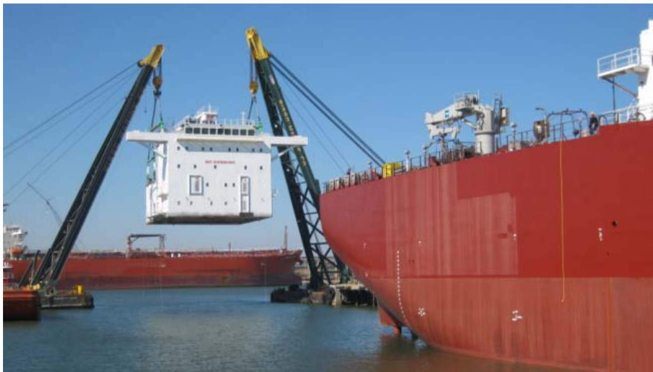
"BISSO MARINE's D/B CAPPY BISSO and D/B LILI BISSO setting a 750 ton superstructure on a newly built US Flagged ship" - Photo courtesy of David Quintero
