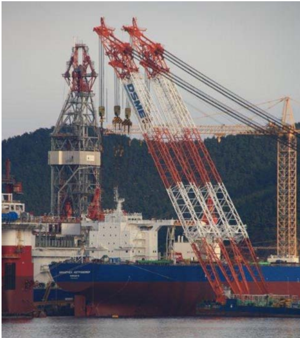
The recently launched vessel ANANGEL ASTRONOMER seen at DSME shipyard receiving her deck house. (Ref : news clipping 305-01-11-2011)
