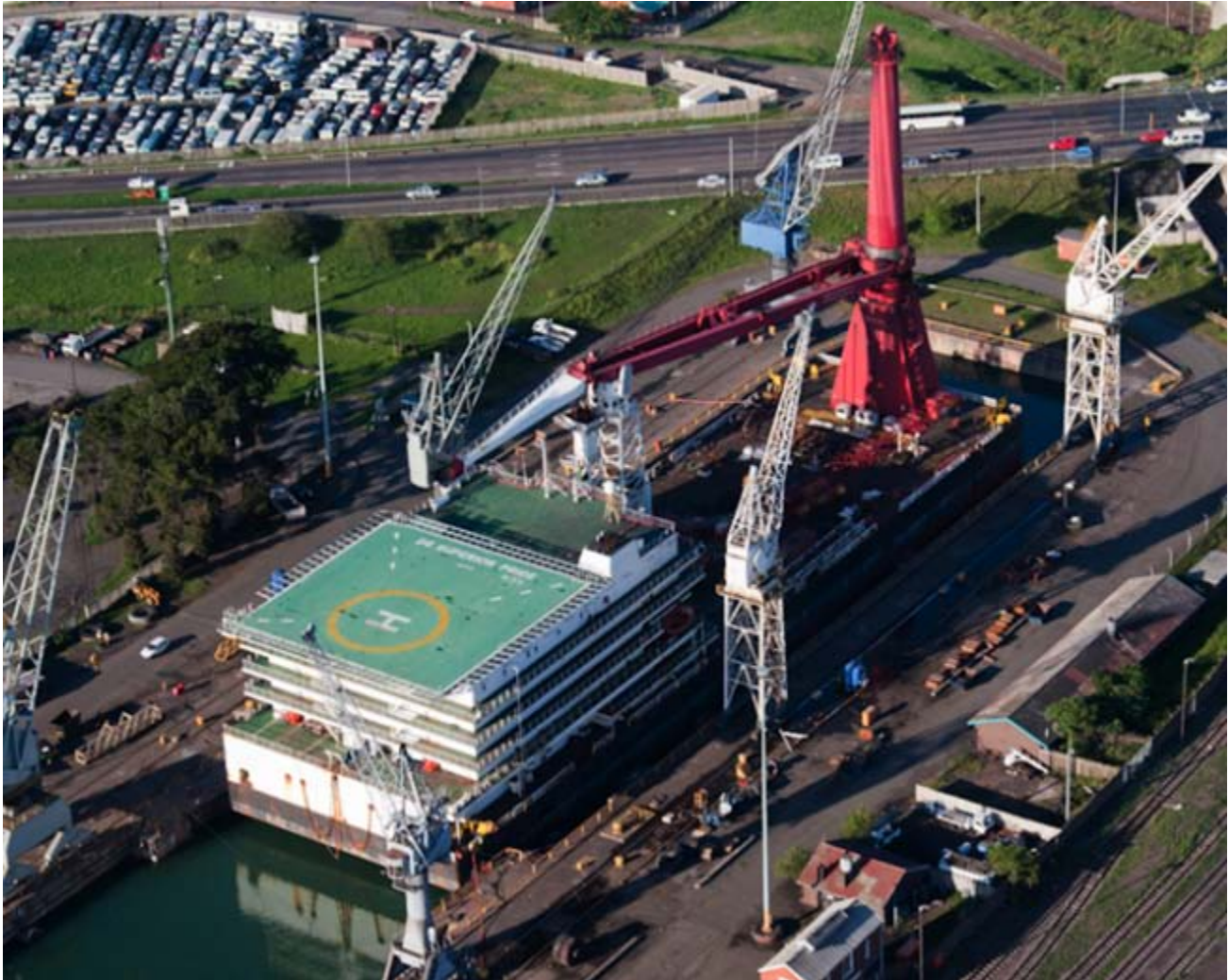
Derrick Barge Superior Pride (800tons SWL derrick and Accommodation for 300 persons) under refit by Elgin Brown and Hamer Durban South Africa.
