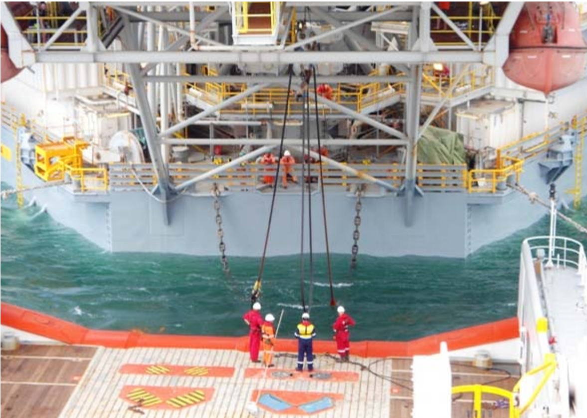
The 28,000 BHP Deep Sea 1 AHTS seen hooking up and towing the Ensco 104 from Singapore headed to Australia. Photo : GO Offshore's Master, Capt. Andrew Malec - submitted by Steve Clark - M3 Marine Group Pte Ltd.
