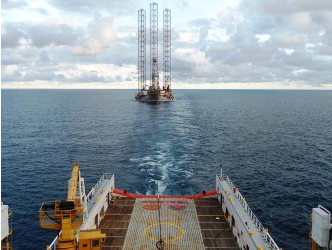
The 28,000 BHP Deep Sea 1 AHTS seen hooking up and towing the Ensco 104 from Singapore headed to Australia. Photo : GO Offshore's Master, Capt. Andrew Malec - submitted by Steve Clark - M3 Marine Group Pte Ltd.
