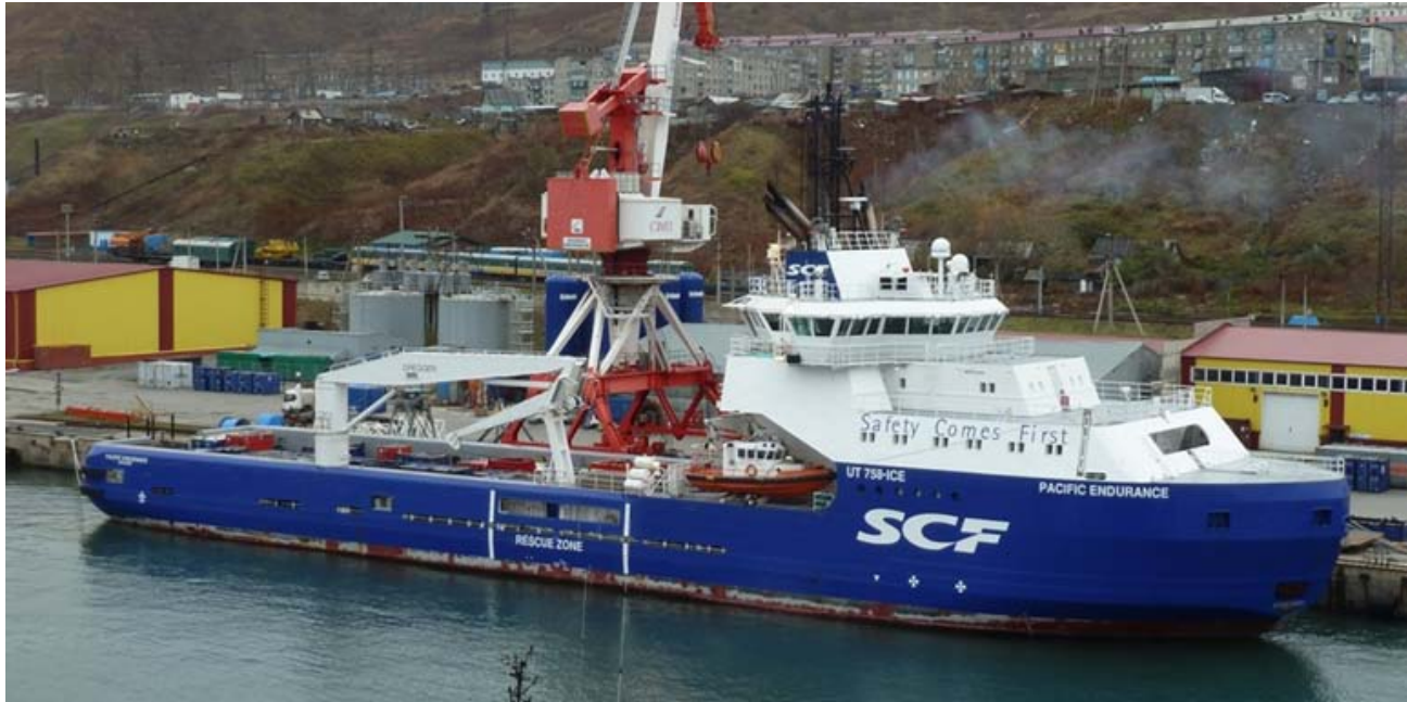
Seen in Kholmsk (Sakhalin) the IBSV Pacific Endurance which can operate in 4 mtr Polar pack ice.
