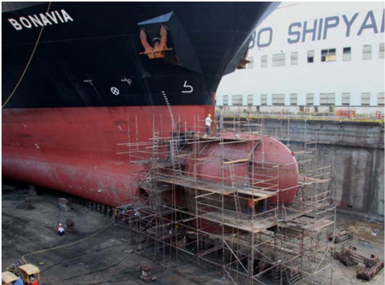
Above seen the 1995 built LBR flag container ship BONAVIA currently drydocked at the Palumbo Malta Shipyard Ltd Dock no 4 with bulbous bow repairs on Tuesday 25th October, 2011.
