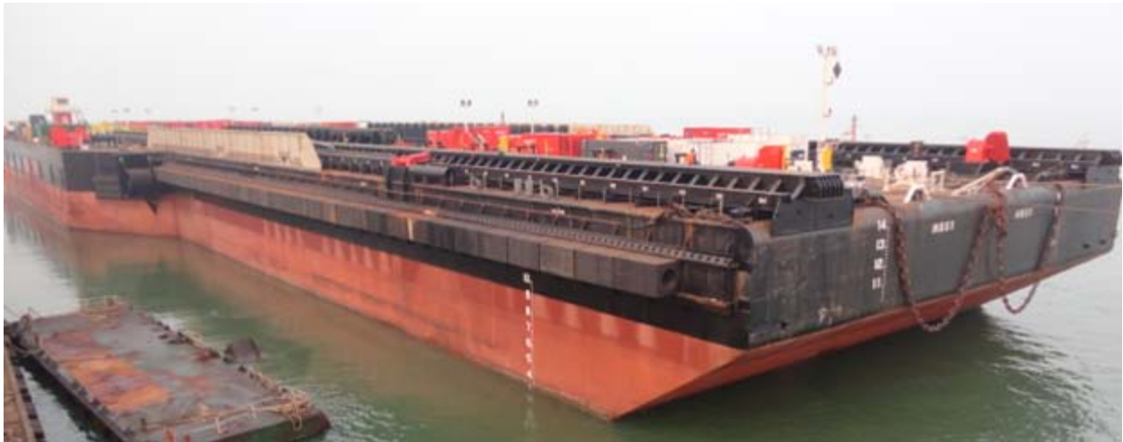
On October 22nd de H-851 left the Yiu Lian yard in Shekou, China after 387 days of conversions and outfitting from a launch barge into a launch and float-over barge. Near Hong Kong Heerema's Husky connected for the offshore tow to Ulsan, Korea. Photo : Willem van Woercom ©
