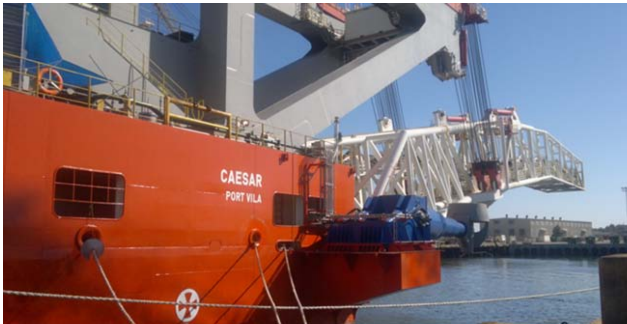
DPPLV Caesar seen in Mobile upgraded with 2x Caterpillar GenSets, 2x Rolls Royce bottom thrusters and 2x Thrustmasters for increased pipelay tension. Photo : Remmelt J. Heemskerk - The Offshore Partners (c)
