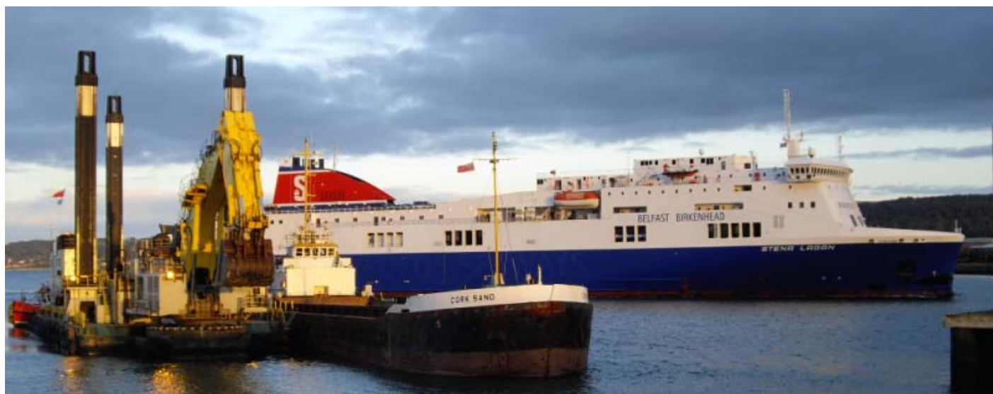
Above seen the Boskalis Backhoe dredger " Nordic Giant " working with the Split hopper barge " Cork Sand " on Stena line's Victoria Terminal 4 extension works. In the background the Stena Lagan just entering the port arriving from Liverpool. - Photo : Jos Verduin (c)
