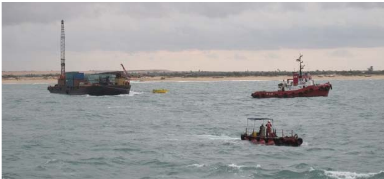
Flat barge "Comarco C231" entering the Exposed Beach Operating System (EBOS) in Moma Sands Mining project , Mozambique carrying 148 mining pontoons and equipment for delivery across the exposed beach.
