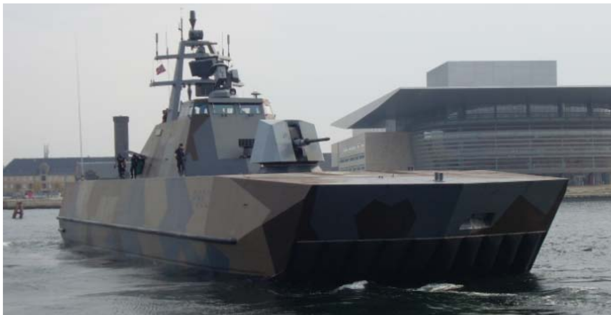
The 2010 delivered Norwegian Navy vessel “ SKUDD ” seen leaving Copenhagen port. The vessel is powered by two Gasoil turbine driving two water jet for a maximum speed of 60 Knots - photo : Lossie M (c)
