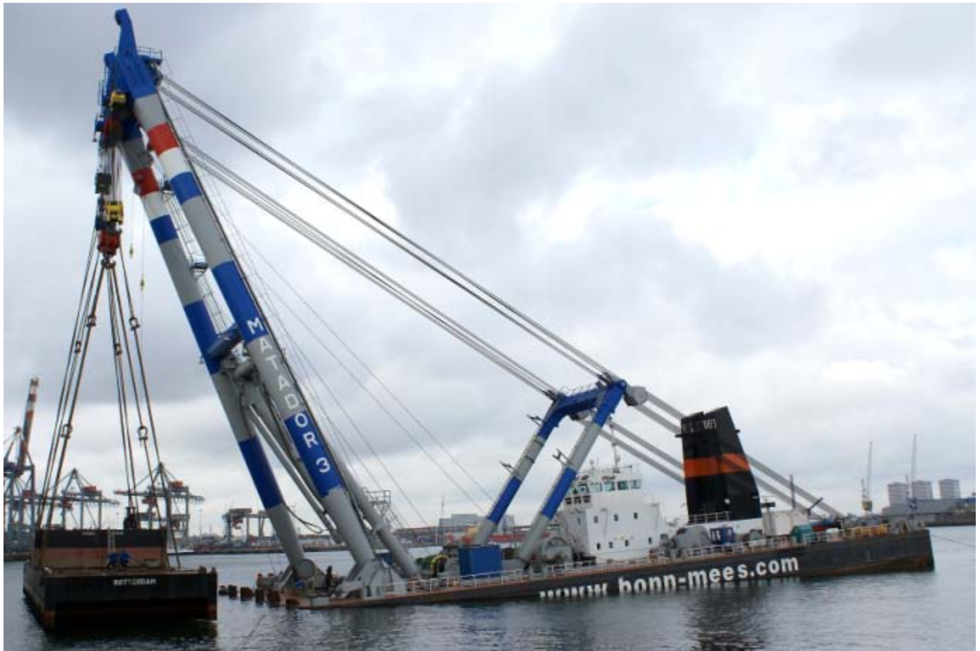
The 1980 tons testlift of the Bonn & Mees floating sheerlegs "Matador 3". The sheerlegs' capacity is now upgraded from 1500 tons to 1800 tons. Photo: Jan Pollemans ©
