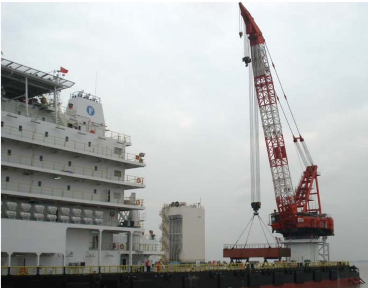
Above seen the 200 pax accommodation/workbarge FRANKLIN VICTORY conducting the lifting test with the 250 tons crane. Photo : FRANKLIN OFFSHORE
